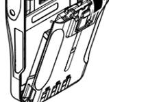
**2** To remove the battery pack, push the lock lever up, then pull the battery pack away from the transceiver.
