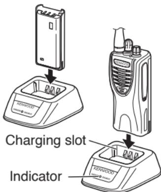
**3** Slide a battery pack or a transceiver equipped with a battery pack into the charging slot of the charger.
