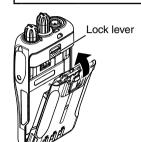
To install the battery pack, align the base of the battery pack with the transceiver, then press the battery pack into place until the lock lever is secure.
